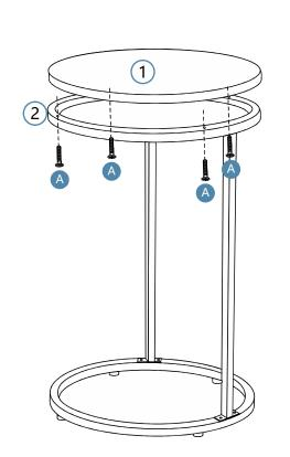
Attach panel [1] to frame [2] with 4 × screws (A).
